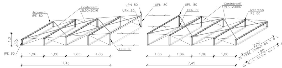
(ASSEMBLAGGIO DI DUE MODULI PESO TOTALE 3.40t)
