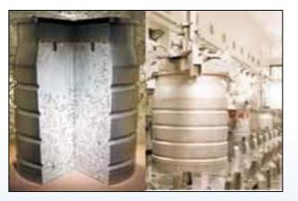
ILW packed in cemented steel drum
